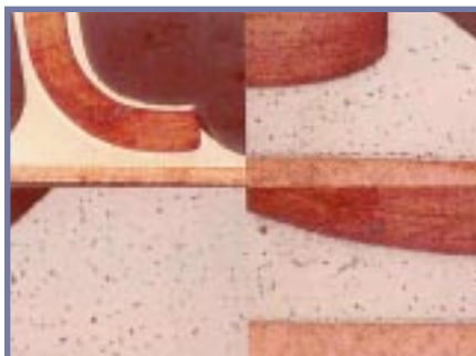
FIGURE 3: Comparison of cross sections of Sn37Pb-soldered (left) and Sn3.8Ag0.7Cu-soldered (right) tin-lead-coated 16-mil pitch QFP component on OSP-coated board.
