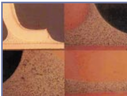
FIGURE 3: Comparison of cross sections of Sn37Pb-soldered (left) and Sn3.8Ag0.7Cu-soldered (right) tin-lead-coated 16-mil pitch QFP component on OSP-coated board.
